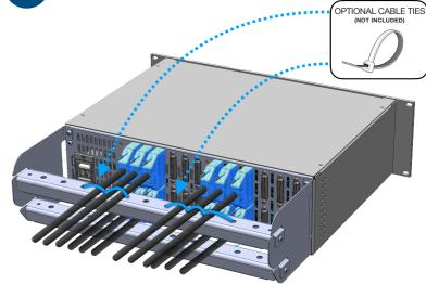
CONNECT & INSTALL ALL DB-25/D-SUB CABLE CONNECTORS TO THE REAR **PATCH**XT PANEL **BEFORE** INSTALLING THE CROSSBARS
